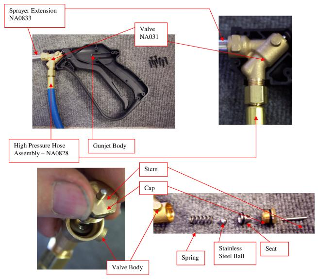
• Examine the Spring, Seat and Steel Ball for signs of wear or pitting. Replace Spring as needed. Replace the Seat o-ring. Replace Steel Ball as needed. Remove Stem from Cap and replace seals as needed. If the valve body or seat is worn or damaged, replace the whole valve (NA031).
